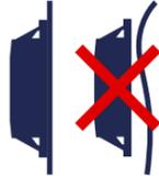
Make sure the mounting surface is **flat and clean**, for a strong and durable bond.
