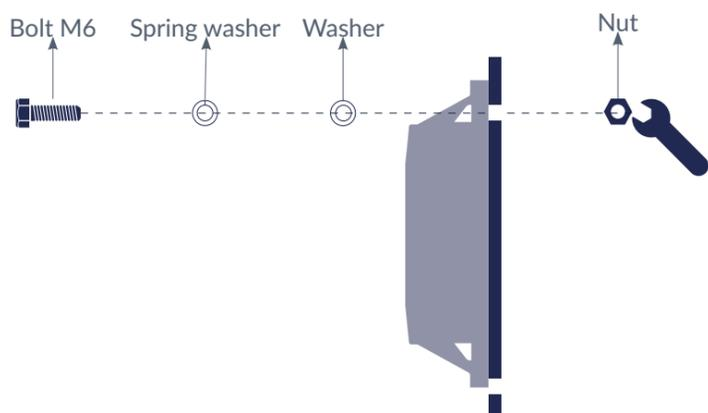
1. Use the appropriate size of screws, it is recommended to use the M6 type and to use thread locking glue on the bolts. We recommend Loctite Thread Locker Blue 242.
